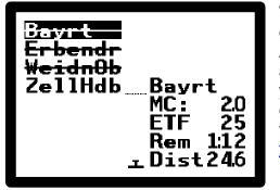
When you start, the start point is automatically crossed off (a line is drawn through the name). As you fly the task, each turnpoint you achieve is automatically crossed off; the picture at left shows you during a task after achieving Weiden and enroute to Zell. Finally, when you finish the task, the finish point is crossed off. <u>See the Task Rules page</u> to learn about automatic start, turnpoint, and finish.
