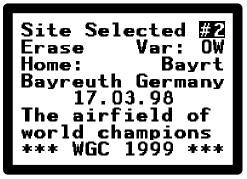
the SN10, including loading a new site description from a PC. The text in the lower part of the screen is the description of the selected site, loaded from a PC.
